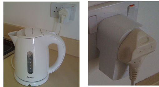
Figure 4. Appliance-level sensing with the Plugwise Zigbee sensor network.
