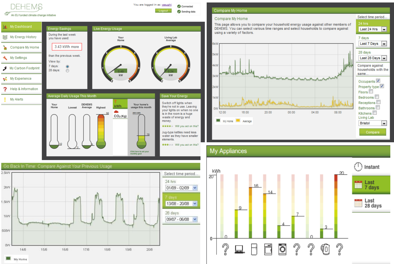
Figure 5. Clockwise from top left: (1) Cycle 2 Dashboard with live energy usage of the home and the Living Lab, comparisons against lowest, average and highest usage in the Living Lab homes and energy saving tips. (2) Comparison against homes fitting a selection of criteria. (3) Individual appliance real-time, weekly and monthly consumption. (4) Historical daily, weekly and monthly power usage.
