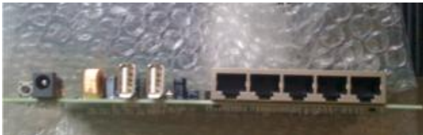
Figure 13 Back of data gateway board showing available ports.
